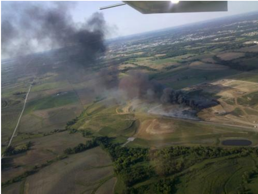
Figure 6.1 Photograph of the Iowa City landfill fire, with smoke primarily from the burning shredded tire drainage layer (Photo courtesy- Thomas Peters)
