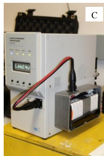
Figure 3.3 Overview of the configuration, assembly, and testing of the mobile CPC. 3.3 A is a schematic configuration in the mobile CPC showing electrical (magenta) and data lines (blue). 3.3 B shows the assembly of the mobile unit in a Pelican case showing integrated GPS, data logger and NiMh battery pack; 3.3 C illustrates the design of the external VDC supply to the CPC 3786.
