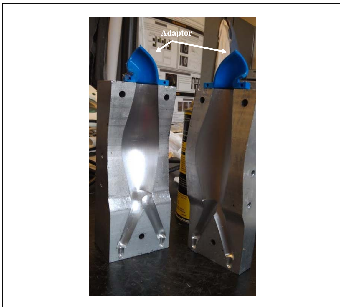
Figure 23: Blue adapters are connected to aluminum mold to allow for creation of different neck angles while using the same AAA body.
