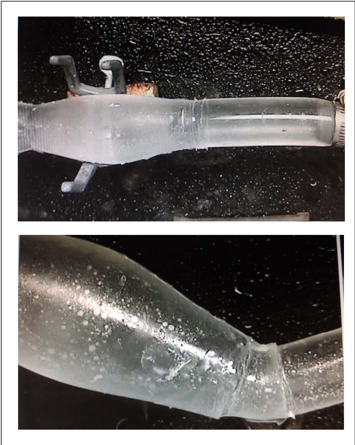
Figure 25: Finished silicone aorta-AAA complex connected into the flow loop. The top picture shows a model with 0^\circ neck angle and bottoms shows 30^\circ .
